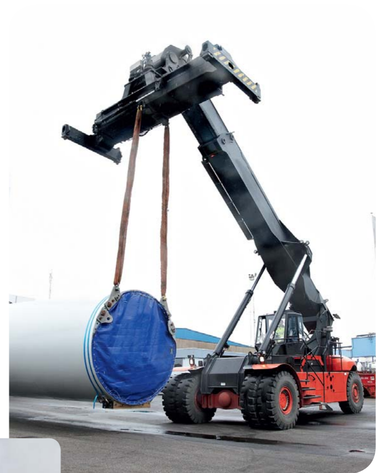
REACHSTACKER handling a tower section.
