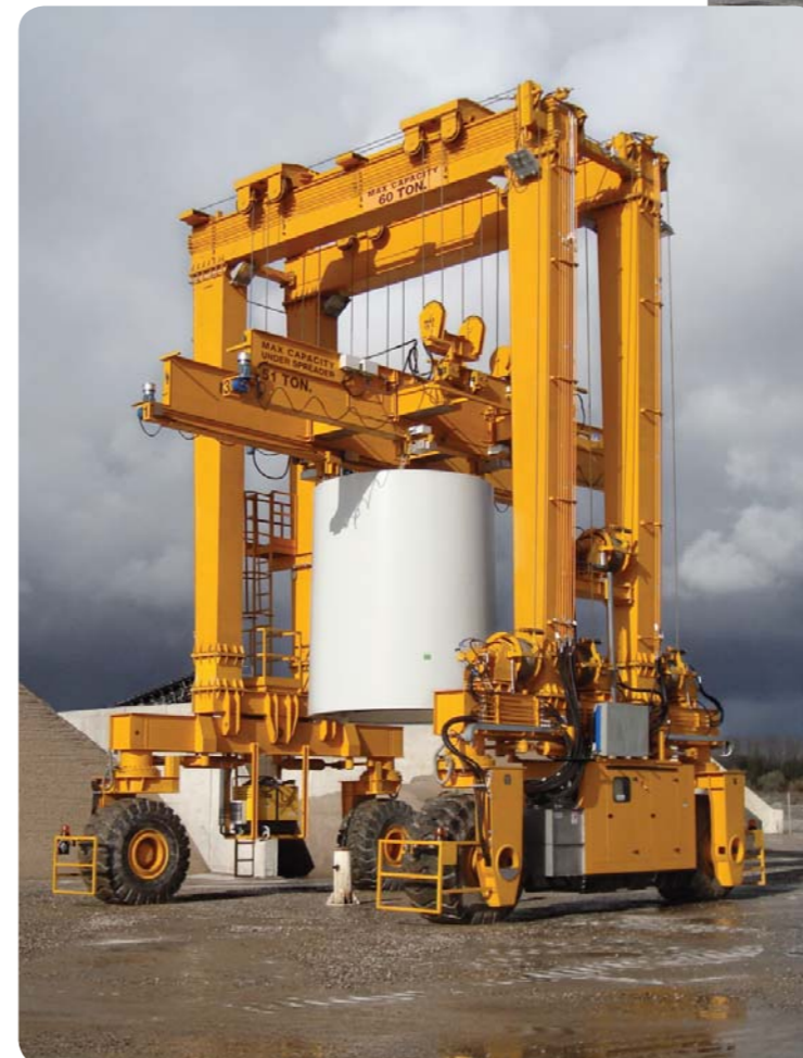
RTG handling a tower section.
