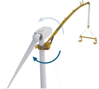
Rotor is turned 120 deg CCW or CW with turning tool while hook is lowered for next blade.
